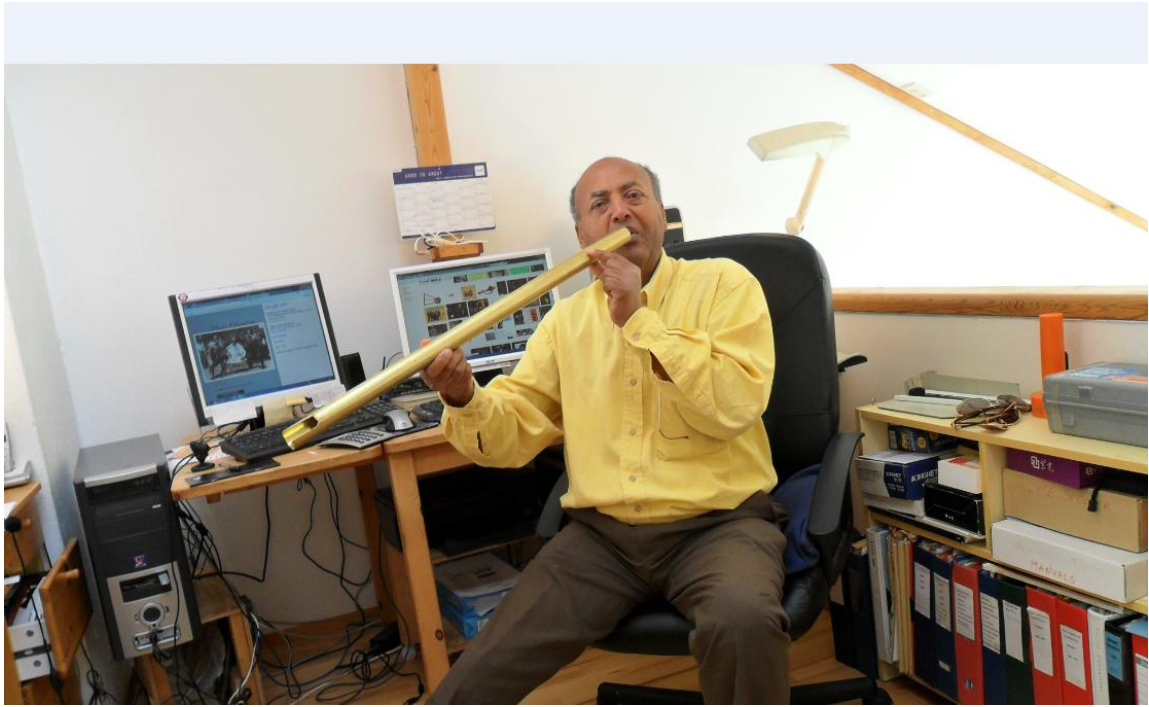
Testing a 110 cm long and 2.5 cm diameter bronze tube with the upper end partly opened
