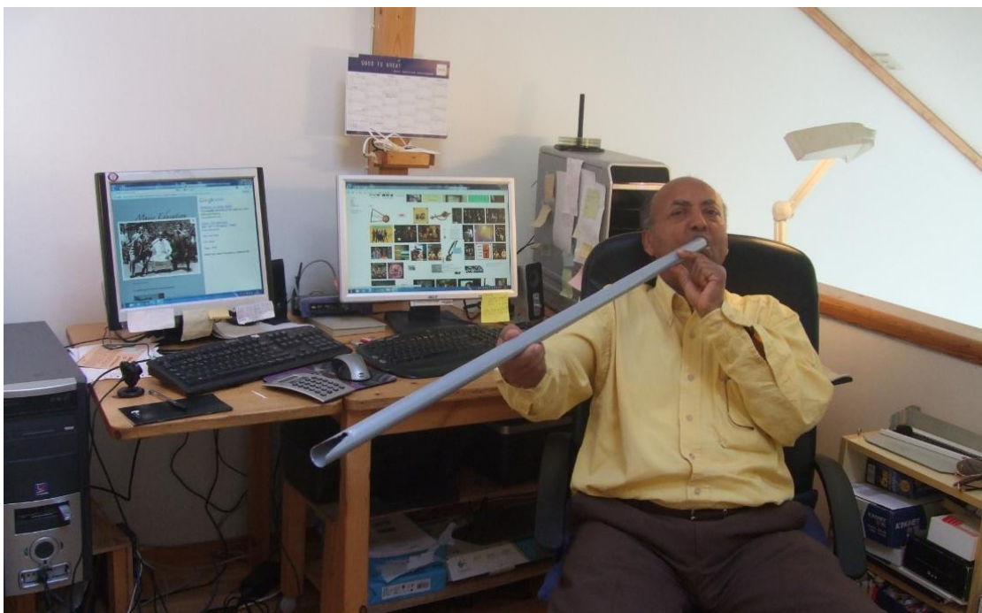
Testing a 140 cm long and 2.5 cm diameter metal tube with the upper end partly opened
